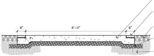
6" PORTLAND CEMENT CONCRETE WITH INTEGRAL MINERAL OXIDE COLORING AGENT. SEE CONCRETE MIX BELOW. LIGHT BROOM FINISH PERPENDICULAR TO TRAFFIC.
