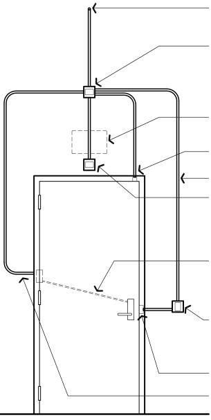
1" CONDUIT. ROUTE TO VOICE/DATA PATHWAY (J-HOOKS OR CABLE TRAY) AND TERMINATE WITH BUSHING.
