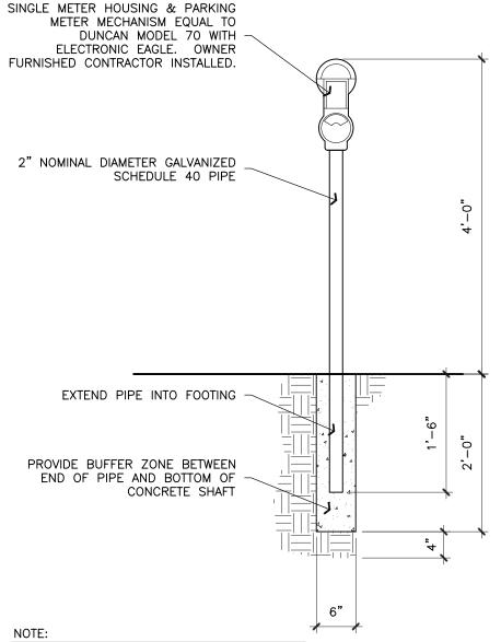
WHERE MORE THAN ONE METER IS TO BE INSTALLED IN A ROW, THE TOPS AS WELL AS THE FACE OF ALL METERS SHALL BE ALIGNED. WHERE NECESSARY SET THE FIRST AND LAST METER IN A ROW AND PULL A STRING BETWEEN THE METERS TO ESTABLISH THE PROPER ALIGNMENT. MINIMUM 48" FROM FINISH GRADE TO TOP OF METER.
