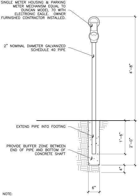
WHERE MORE THAN ONE METER IS TO BE INSTALLED IN A ROW, THE TOPS AS WELL AS THE FACE OF ALL METERS SHALL BE ALIGNED. WHERE NECESSARY SET THE FIRST AND LAST METER IN A ROW AND PULL A STRING BETWEEN THE METERS TO ESTABLISH THE PROPER ALIGNMENT. MINIMUM 48" FROM FINISH GRADE TO TOP OF METER.
