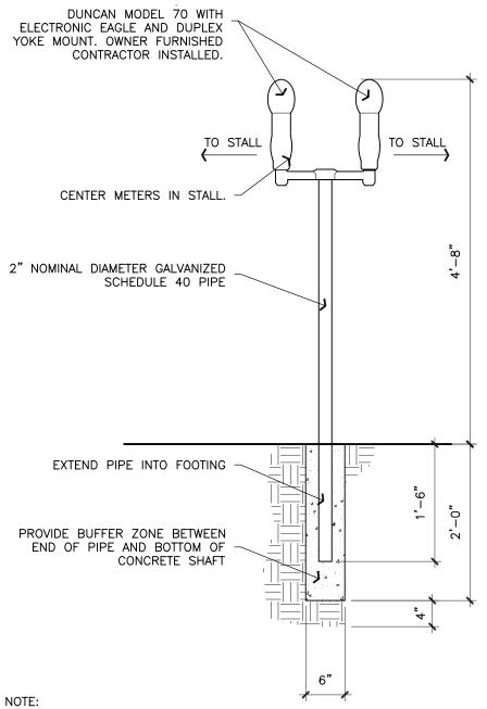
WHERE MORE THAN ONE METER IS TO BE INSTALLED IN A ROW, THE TOPS AS WELL AS THE FACE OF ALL METERS SHALL BE ALIGNED. WHERE NECESSARY SET THE FIRST AND LAST METER IN A ROW AND PULL A STRING BETWEEN THE METERS TO ESTABLISH THE PROPER ALIGNMENT. MINIMUM 48" FROM FINISH GRADE TO TOP OF METER.
